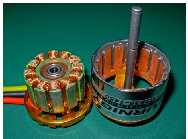
Outrunner Brushless Motor: (Left) Stator, (Right) permanent magnets fixed to the bell
